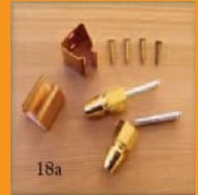
The bullet catch is designed to go behind the shutter, in the open position typically on the back of the side stile furthest from the window. The bullet or acorn shaped piece is fixed to the house and the locking catch or receiver is screwed to the shutter and catches the bullet holding the shutter in the open position. Bullet catches are made of brass and sold in two styles; one for masonry construction and one for lap types of siding such as wood, fiber cement, vinyl, etc.
